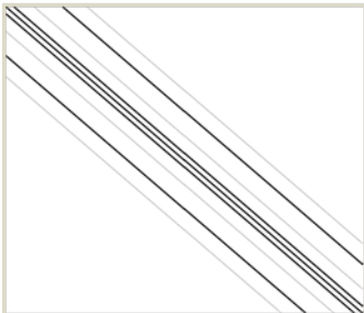
Fig. 1: The sparse Matrix: White areas have zero values, thick lines are 3 diagonals in a row and thin lines are single diagonals.
